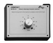
For instance if the source is a generator of 2000 Watt, the potentiometer has to be set at max. 8A. This value is obtained in dividing 2000 Watt by 230V. If the COMPACT is connected to a power source which is protected by a 6A circuit breaker, the potentiometer must be set at a max. value of 6A.
