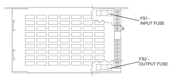
Both the input and output fuses are accessed by removing the cover (held in place by screw 'X'). Both fuses must be replaced by fuses with the same type and rating.
