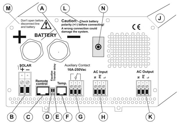
A Battery +/- Battery cable (already installed)
