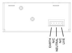
Where installed in a system cabinet, the PSU's earth conductor should not be used as the overall system earth. Cabinets should have supplementary earth bonding in accordance with the installed equipment.
