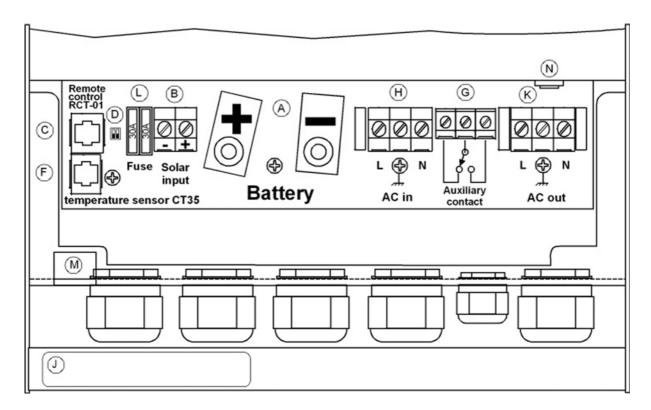
A Battery +/- Connection terminal (M8) for battery cable (HPC 4400-24/6000-
