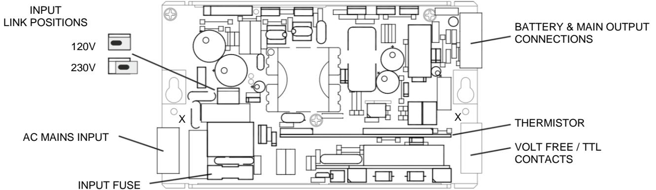
The input fuse is accessed by removing the cover (held in place by two screws 'X'). The fuse must be replaced with the same type and rating. The output fuse is non-replaceable, this is a return to manufacturer replacement part.
