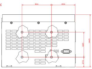
**Mounting information** 4 mounting bushes M3, screws should not penetrate the unit chassis by more than 5mm.
