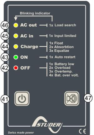
The table below describes the type of fault according to the number of flashes on the indicator (42)
