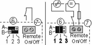
In multi-unit configurations (see below) the chosen functionality must be the same in every unit in the system. Only one unit can be wired to apply the function to every Xtender in the system. If the entry command is used as an emergency stop, (all functions halted) it have t be wired on the unit with the highest serial number (master).
