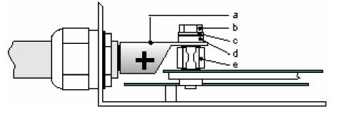
a = bolt M8 x 30) b = washer c = ceramic washer
