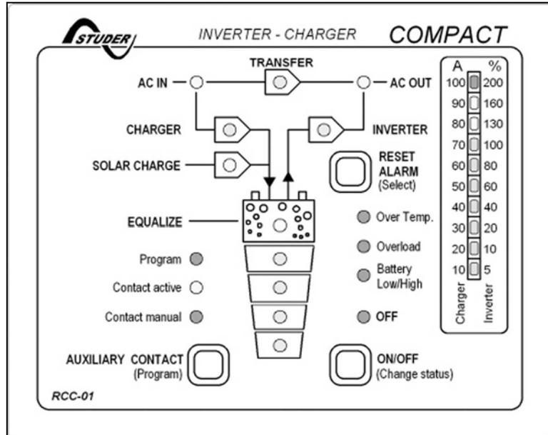
The output power and the charging currents are displayed on the Remote Control. In the Remote Control there is an additional Alarm Contact and a built-in Control Input. These two functions are available through Tip-jack RJ11/4 for use. This Auxiliary Contact is Front / Work Contact (max. 0.5A!), which is independent from the Auxiliary Contact of the HP-COMPACT. This contact is active in case of an alarm of the HP-COMPACT.
