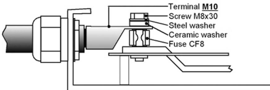
The supplied fuse (except with the HPC 2800-12) must be mounted according to the plan below.
