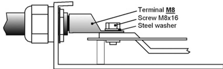
Connect the black cable (-) on the “- Battery” appliance connection point according to the plan above.
