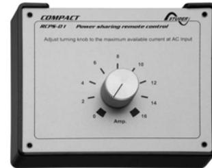
For instance if the source is a generator of 2000 Watt, the potentiometer has to be set at max. 8A. This value is obtained in dividing 2000 Watt by 230V. If the HP-COMPACT is connected to a power source which is protected by a 6A circuit breaker, the potentiometer must be set at a max. value of 6A.
