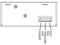
Where installed in a system cabinet, the psu earth conductor should not be used as the overall system earth. Cabinets should have supplementary earth bonding in accordance with the installed equipment.
