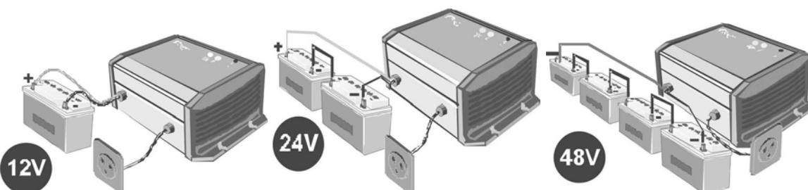
The cable of the battery is supplied with the inverter and already connected in it. A fuse must be installed on the battery. Connect the battery observing carefully the polarity. The AJ inverter, **AJ 2100-12**, is protected against inversion by a fuse, but if the polarity should be inverted, the inverter must be sent to the manufacturer for control.
